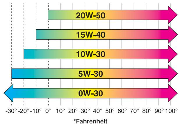
**Viscosity improvers** are viscous chemical compounds called polymers or polymeric compounds that decrease the rate at which oils change viscosity with temperature. Viscosity improvers extend a motor oil's operating temperature range and allow the manufacture of multi-grade or all-season oils. Low-quality viscosity improvers, however, lend themselves to shearing.
