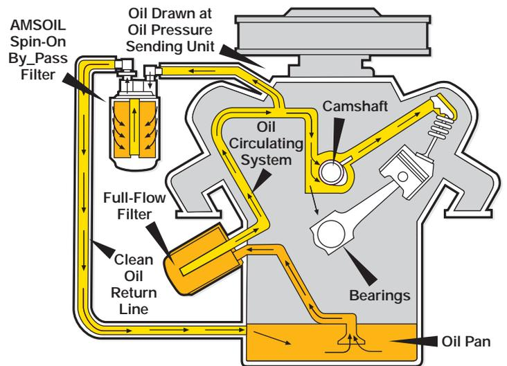
By-pass filters operate by filtering oil on a “partial-flow” basis. They draw approximately 10 percent of the oil pump’s capacity at any one time and trap the extremely small, wear-causing contaminants that full-flow filters can’t remove. The continual process eventually makes all the oil analytically clean, reducing long-term wear and helping extend oil life.
